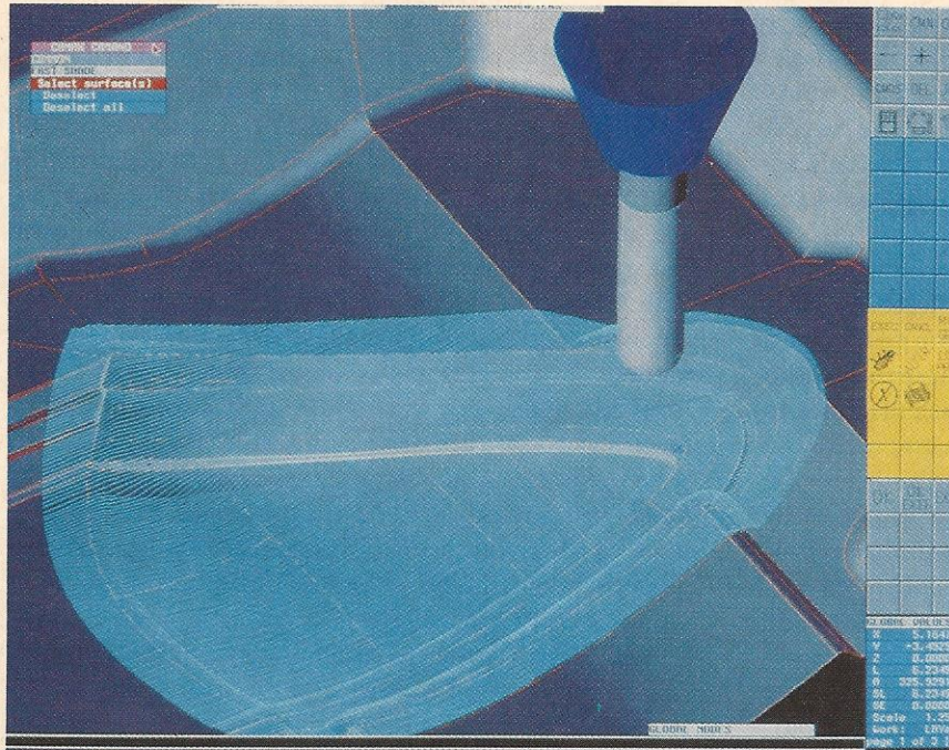
Computer-aided manufacturing software can handle many disparate functions in an integrated way that formerly required separate activities. The Camand system from Camax Systems Inc. can be used to model, render, and create five-axis tool paths for parts. Pictured here is a close-up view of an automotive taillight mold cavity composed of 260 surfaces rendered in Camand's Viewmax module. The image displays the mold cavity, parting-line surfaces, and tool paths.
